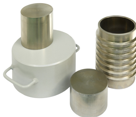
Mold, upper and lower stamps, and weight for Ø71.4 mm mold
