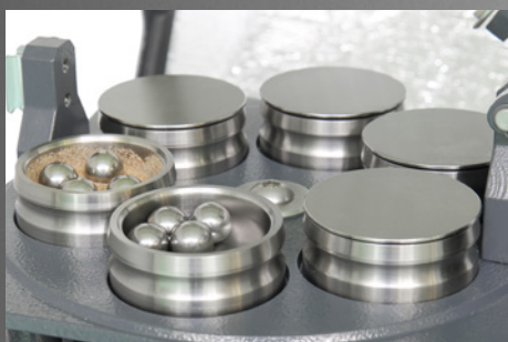
Platform of VG 6 with cups and fastener
