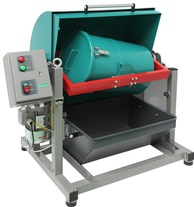
Shaker mixer SM 50.0 «Drum Tumbler», drum tilt angle – 15°
