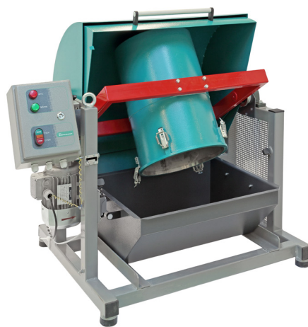
Shaker mixer SM 50.0 «Drum Tumbler» in "Unloading" position
