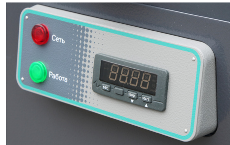
Built-in control panel with timer
