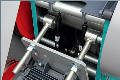
Device for adjusting tension of electric motor belts on JC 15
