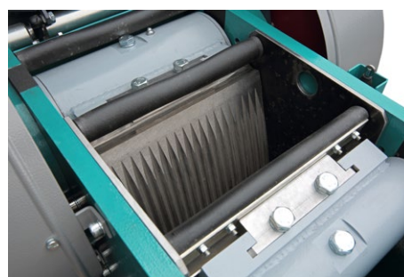
Crank arm, armor, jaws and jaw fastening wedge of JC 15
