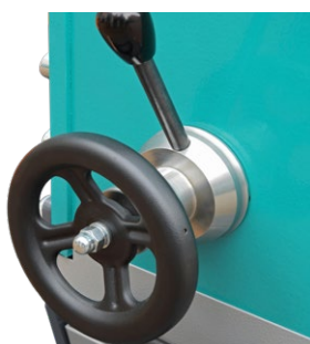
Device for adjusting gap between jaws of JC 15
