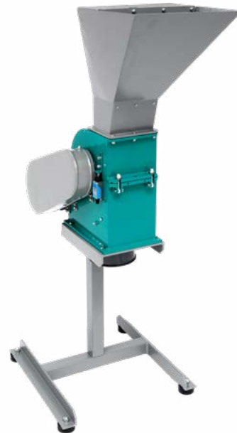
Hammer crusher HC 2x2
