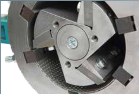
CM 120 working chamber (rotor, blades, discharge grate)
