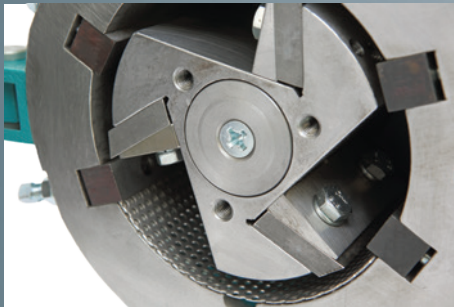
CM 120 working chamber (rotor, blades, discharge grate)
